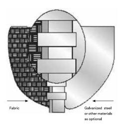
The double flanged seam gives an exceptional strength to the connection between steel and fabric. The above seam is used in all our duct connectors.
